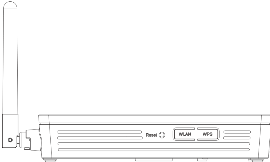
Figure 1-4 Ports and buttons on the side cover of the HG8245H
