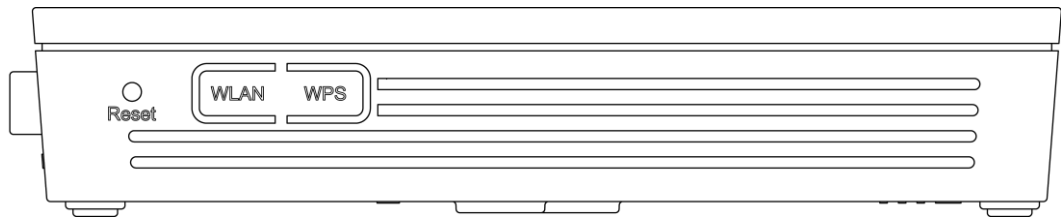
Figure 1-9 Ports and buttons on the side cover of the HG8045A
